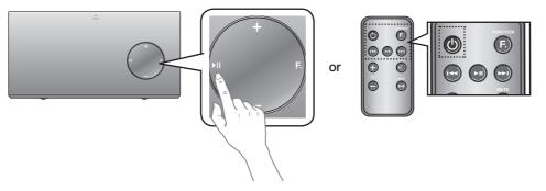
1. To turn on this unit, press any button on the unit's top panel when the unit is in Standby mode.
